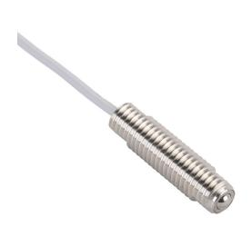
Metrol limit switch, precision touch, 10mm diameter, threaded, 1.5mm pitch, 33mm length, 5mm head, stainless steel, ball plunger, 1N contact force, N.O. contact(s), 6.5ft/2m cable length, pigtail.
