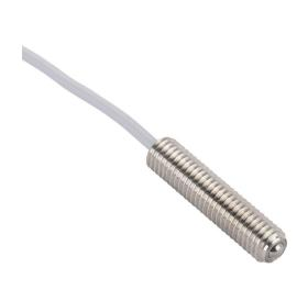
Metrol limit switch, precision touch, 8mm diameter, threaded, 1.25mm pitch, 30mm length, 4mm head, stainless steel, ball plunger, 1N contact force, N.O. contact(s), 6.5ft/2m cable length, pigtail.
