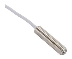
Metrol limit switch, precision touch, 8mm diameter, threaded, 1.25mm pitch, 30mm length, 4mm head, stainless steel, ball plunger, 1N contact force, (1) N.O. contact(s), 6.5ft/2m cable length, pigtail.
