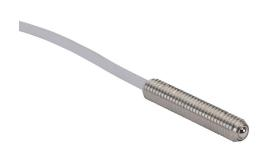
Metrol limit switch, precision touch, 6mm diameter, threaded, 1mm pitch, 32.8mm length, 3mm head, stainless steel, ball plunger, 8-13N contact force, N.O. contact(s), 6.5ft/2m cable length, pigtail.
