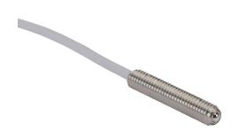
Metrol limit switch, precision touch, 6mm diameter, threaded, 1mm pitch, 32.8mm length, 3mm head, stainless steel, ball plunger, 8-13N contact force, (1) N.O. contact(s), 6.5ft/2m cable length, pigtail.
