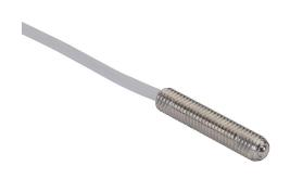
Metrol limit switch, precision touch, 6mm diameter, threaded, 1mm pitch, 32.8mm length, 3mm head, stainless steel, ball plunger, 1N contact force, N.O. contact(s), 6.5ft/2m cable length, pigtail.
