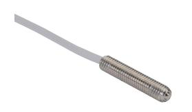
Metrol limit switch, precision touch, 6mm diameter, threaded, 1mm pitch, 32.8mm length, 3mm head, stainless steel, ball plunger, 1N contact force, (1) N.O. contact(s), 6.5ft/2m cable length, pigtail.
