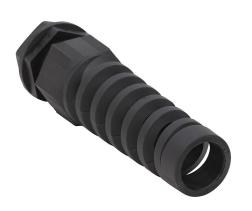
Bimed cable gland, 3/4in NPT thread type, polyamide, black, accepts 13 to 18mm diameter cable, IP68, with strain relief. Package of 5. Mounting hardware included.
