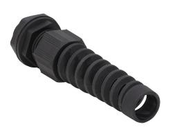
Bimed cable gland, 1/2in NPT thread type, polyamide, black, accepts 6 to 12mm diameter cable, IP68, with strain relief. Package of 5. Mounting hardware included.
