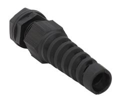
Bimed cable gland, 3/8in NPT thread type, polyamide, black, accepts 5 to 10mm diameter cable, IP68, with strain relief. Package of 5. Mounting hardware included.
