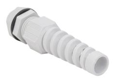
Bimed cable gland, 3/8in NPT thread type, polyamide, light gray, accepts 5 to 10mm diameter cable, IP68, with strain relief. Package of 5. Mounting hardware included.
