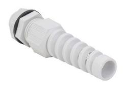
Bimed cable gland, 3/8in NPT thread type, polyamide, light gray, accepts 5 to 10mm diameter cable, IP68, with strain relief. Package of 5. Mounting hardware included.
