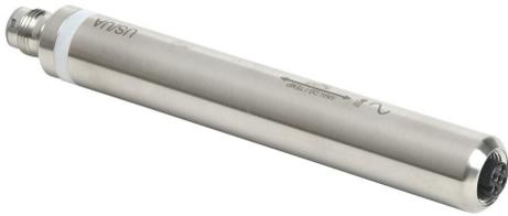
Balluff temperature/analog combo converter, 1-channel, current/voltage/RTD/thermocouple, 16-bit, input RTD type(s): Pt100 and Pt1000, input thermocouple type(s): J, K, IO-Link v1.1, stainless steel housing, IP65 and IP67. Requires IO-Link master.
