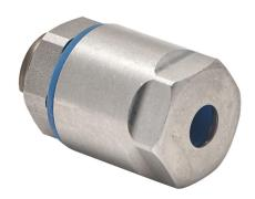
Bimed hygienic cable gland, 1/4in NPT thread type, stainless steel, accepts 3 to 6.5mm diameter cable, IP66, IP68 and IP69. Mounting hardware included. Allen wrench size 7mm, use adapter BMFGT-01 to reduce Allen wrench size to 5mm.
