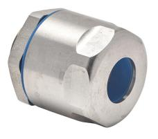
Bimed hygienic cable gland, 3/4in NPT thread type, stainless steel, accepts 12 to 17mm diameter cable, IP66, IP68 and IP69. Mounting hardware included. Allen wrench size 17mm, use adapter BMFGT-04 to reduce Allen wrench size to 10mm.
