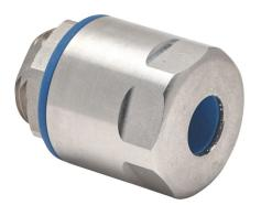
Bimed hygienic cable gland, 1/2in NPT thread type, stainless steel, accepts 6 to 12mm diameter cable, IP66, IP68 and IP69. Mounting hardware included. Allen wrench size 13mm, use adapter BMFGT-03 to reduce Allen wrench size to 8mm.
