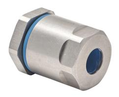
Bimed hygienic cable gland, 3/8in NPT thread type, stainless steel, accepts 5 to 10mm diameter cable, IP66, IP68 and IP69. Mounting hardware included. Allen wrench size 10mm, use adapter BMFGT-02 to reduce Allen wrench size to 6mm.
