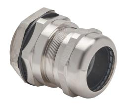
Bimed EMC cable gland, 2in NPT thread type, nickel-plated brass, accepts 34 to 44mm diameter cable, IP68. Mounting hardware included.
