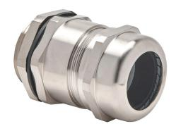
Bimed EMC cable gland, 1-1/2in NPT thread type, nickel-plated brass, accepts 30 to 38mm diameter cable, IP68. Mounting hardware included.
