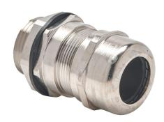
Bimed EMC cable gland, 1in NPT thread type, nickel-plated brass, accepts 16 to 25mm diameter cable, IP68. Package of 5. Mounting hardware included.
