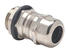
Bimed EMC cable gland, 3/4in NPT thread type, nickel-plated brass, accepts 10 to 18mm diameter cable, IP68. Package of 5. Mounting hardware included.
