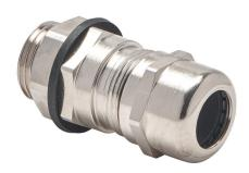
Bimed EMC cable gland, 1/2in NPT thread type, nickel-plated brass, accepts 7.5 to 14mm diameter cable, IP68. Package of 5. Mounting hardware included.
