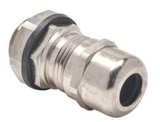
Bimed EMC cable gland, 3/8in NPT thread type, nickel-plated brass, accepts 5 to 10mm diameter cable, IP68. Package of 5. Mounting hardware included.
