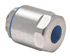
Bimed hygienic EMC cable gland, 3/4in NPT thread type, stainless steel, accepts 12 to 17mm diameter cable, IP66, IP68 and IP69. Mounting hardware included. Allen wrench size 17mm, use adapter BMFGT-04 to reduce Allen wrench size to 10mm.
