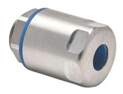
Bimed hygienic EMC cable gland, 1/2in NPT thread type, stainless steel, accepts 6 to 12mm diameter cable, IP66, IP68 and IP69. Mounting hardware included. Allen wrench size 13mm, use adapter BMFGT-03 to reduce Allen wrench size to 8mm.
