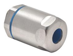
Bimed hygienic EMC cable gland, 3/8in NPT thread type, stainless steel, accepts 5 to 10mm diameter cable, IP66, IP68 and IP69. Mounting hardware included. Allen wrench size 10mm, use adapter BMFGT-02 to reduce Allen wrench size to 6mm.
