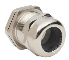
Bimed cable gland, 1in NPT thread type, nickel-plated brass, accepts 18 to 25mm diameter cable, IP68. Package of 5. Mounting hardware included.
