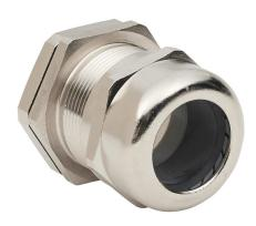
Bimed cable gland, 1in NPT thread type, nickel-plated brass, accepts 18 to 25mm diameter cable, IP68. Package of 5. Mounting hardware included.
