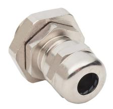
Bimed cable gland, 3/8in NPT thread type, nickel-plated brass, accepts 4 to 8mm diameter cable, IP68. Package of 5. Mounting hardware included.
