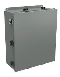
Wiegmann enclosure, NEMA 4/12/13,  $16 \times 14 \times 6$  in (HxWxD), wall mount, carbon steel, ANSI 61 gray, powder coat finish, lift-off cover, (10) stainless steel clamps.
