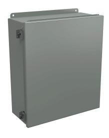
Wiegmann enclosure, NEMA 4/12/13, 16 x 14 x 6in (HxWxD), wall mount, carbon steel, ANSI 61 gray, powder coat finish, singledoor, (2) stainless steel clamps.
