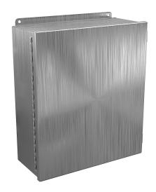
Wiegmann enclosure, NEMA 4/4X/12/13, 16 x 14 x 6in (HxWxD), wall mount, 304 stainless steel, No. 3 intermediate polished finish, single-door, (2) stainless steel clamps.
