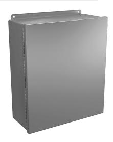
Wiegmann enclosure, NEMA 4/4X/12/13, 16 x 14 x 6in (HxWxD), wall mount, 5052-H32 aluminum, No. 3 intermediate polished finish, single-door, (2) stainless steel clamps.
