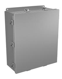
Wiegmann enclosure, NEMA 4/4X/12/13, 16 x 14 x 6in (HxWxD), wall mount, 5052-H32 aluminum, No. 3 intermediate polished finish, lift-off cover, (10) stainless steel clamps.
