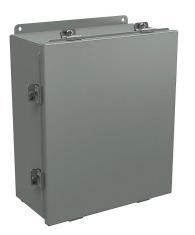
Wiegmann enclosure, NEMA 4/12/13, 14 x 12 x 6in (HxWxD), wall mount, carbon steel, ANSI 61 gray, powder coat finish, lift-off cover, (8) stainless steel clamps.
