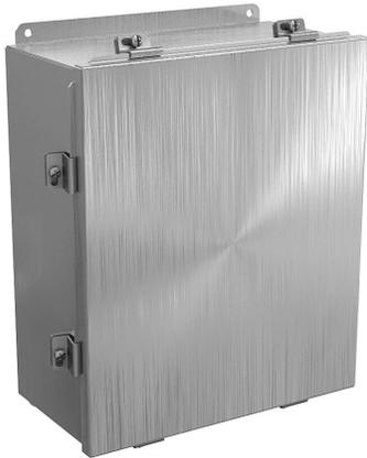
Wiegmann enclosure, NEMA 4/4X/12/13, 14 x 12 x 6in (HxWxD), wall mount, 304 stainless steel, No. 3 intermediate polished finish, lift-off cover, (8) stainless steel clamps.
