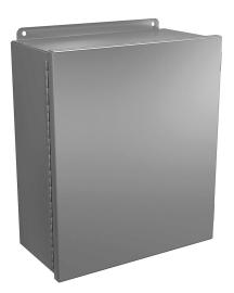
Wiegmann enclosure, NEMA 4/4X/12/13, 14 x 12 x 6in (HxWxD), wall mount, 5052-H32 aluminum, No. 3 intermediate polished finish, single-door, (2) stainless steel clamps.
