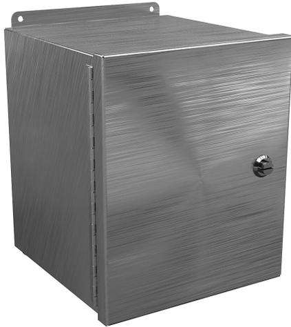
Wiegmann Ultimate Mini-Max series enclosure, NEMA 4/4X/12, 12 x 10 x 10in (HxWxD), wall mount, 304 stainless steel, No. 3 intermediate polished finish, single-door, 1/4-turn semi-flush oil-tight latch.
