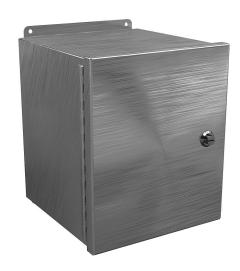
Wiegmann Ultimate Mini-Max series enclosure, NEMA 4/4X/12,  $12 \times 10 \times 10$  in (HxWxD), wall mount, 304 stainless steel, No. 3 intermediate polished finish, single-door, 1/4-turn semi-flush oil-tight latch.
