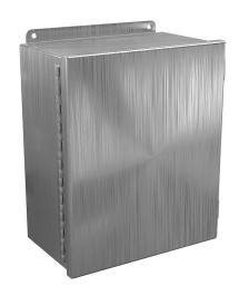
Wiegmann enclosure, NEMA 4/4X/12/13, 12 x 10 x 6in (HxWxD), wall mount, 304 stainless steel, No. 3 intermediate polished finish, single-door, (2) stainless steel clamps.
