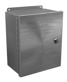
Wiegmann Ultimate Mini-Max series enclosure, NEMA 4/4X/12,  $12 \times 10 \times 6$  in (HxWxD), wall mount, 304 stainless steel, No. 3 intermediate polished finish, single-door, 1/4-turn semi-flush oil-tight latch.
