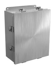
Wiegmann enclosure, NEMA 4/4X/12/13,  $12 \times 10 \times 5$  in (HxWxD), wall mount, 304 stainless steel, No. 3 intermediate polished finish, lift-off cover, (8) stainless steel clamps.
