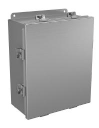
Wiegmann enclosure, NEMA 4/4X/12/13, 12 x 10 x 5in (HxWxD), wall mount, 5052-H32 aluminum, No. 3 intermediate polished finish, lift-off cover, (8) stainless steel clamps.
