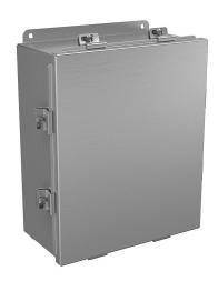
Wiegmann enclosure, NEMA 4/4X/12/13,  $12 \times 10 \times 5$ in (HxWxD), wall mount, 5052-H32 aluminum, No. 3 intermediate polished finish, lift-off cover, (8) stainless steel clamps.
