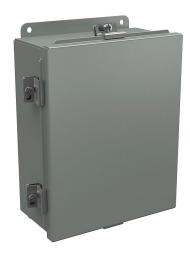
Wiegmann enclosure, NEMA 4/12/13, 10 x 8 x 4in (HxWxD), wall mount, carbon steel, ANSI 61 gray, powder coat finish, lift-off cover, (6) stainless steel clamps.
