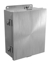
Wiegmann enclosure, NEMA 4/4X/12/13, 10 x 8 x 4in (HxWxD), wall mount, 304 stainless steel, No. 3 intermediate polished finish, lift-off cover, (6) stainless steel clamps.
