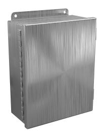
Wiegmann enclosure, NEMA 4/4X/12/13, 10 x 8 x 4in (HxWxD), wall mount, 304 stainless steel, No. 3 intermediate polished finish, single-door, (2) stainless steel clamps.
