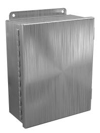
Wiegmann enclosure, NEMA 4/4X/12/13,  $10 \times 8 \times 4$ in (HxWxD), wall mount, 304 stainless steel, No. 3 intermediate polished finish, single-door, (2) stainless steel clamps.
