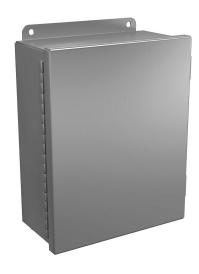
Wiegmann enclosure, NEMA 4/4X/12/13, 10 x 8 x 4in (HxWxD), wall mount, 5052-H32 aluminum, No. 3 intermediate polished finish, single-door, (2) stainless steel clamps.
