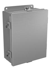
Wiegmann enclosure, NEMA 4/4X/12/13, 10 x 8 x 4in (HxWxD), wall mount, 5052-H32 aluminum, No. 3 intermediate polished finish, lift-off cover, (6) stainless steel clamps.
