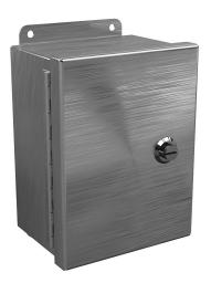
Wiegmann Ultimate Mini-Max series enclosure, NEMA 4/4X/12, 8 x 6 x 4in (HxWxD), wall mount, 304 stainless steel, No. 3 intermediate polished finish, single-door, 1/4-turn semi-flush oil-tight latch.
