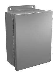
Wiegmann enclosure, NEMA 4/4X/12/13, 8 x 6 x 3in (HxWxD), wall mount, 5052-H32 aluminum, No. 3 intermediate polished finish, single-door, (2) stainless steel clamps.
