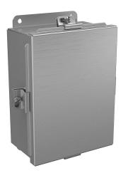
Wiegmann enclosure, NEMA 4/4X/12/13, 8 x 6 x 3in (HxWxD), wall mount, 5052-H32 aluminum, No. 3 intermediate polished finish, lift-off cover, (4) stainless steel clamps.
