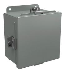
Wiegmann enclosure, NEMA 4/12/13, 6 x 6 x 4in (HxWxD), wall mount, carbon steel, ANSI 61 gray, powder coat finish, lift-off cover, (4) stainless steel clamps.
