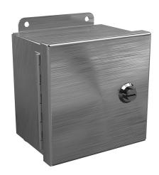
Wiegmann Ultimate Mini-Max series enclosure, NEMA 4/4X/12, 6 x 6 x 4in (HxWxD), wall mount, 304 stainless steel, No. 3 intermediate polished finish, single-door, 1/4-turn semi-flush oil-tight latch.
