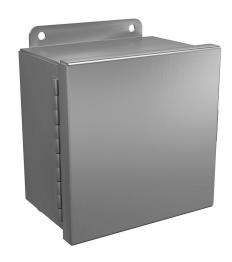
Wiegmann enclosure, NEMA 4/4X/12/13, 6 x 6 x 4in (HxWxD), wall mount, 5052-H32 aluminum, No. 3 intermediate polished finish, single-door, (1) stainless steel clamp.
