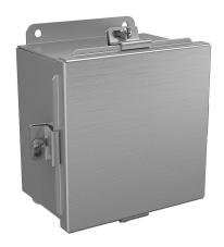
Wiegmann enclosure, NEMA 4/4X/12/13, 6 x 6 x 4in (HxWxD), wall mount, 5052-H32 aluminum, No. 3 intermediate polished finish, lift-off cover, (4) stainless steel clamps.
