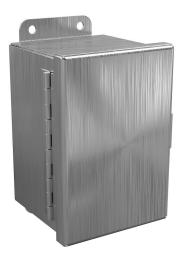
Wiegmann enclosure, NEMA 4/4X/12/13, 6 x 4 x 4in (HxWxD), wall mount, 304 stainless steel, No. 3 intermediate polished finish, single-door, (1) stainless steel clamp.
